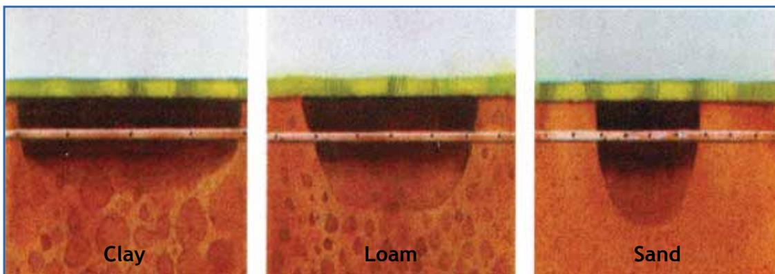
**Figure 4: The influence of soil texture on the wetted width and depth under drip irrigation**
