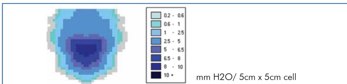
Figure 2: The distribution patterns of water in a soil 48 hours after application when applied from a point source
