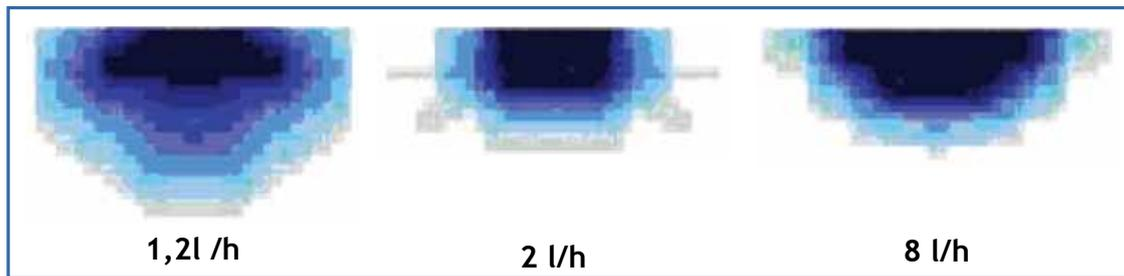
Figure 5a: The water distribution after 50mm application for a different dripper discharge
