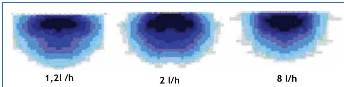
Figure 5b: Water distribution 3 days after 50mm application for a different dripper discharge
