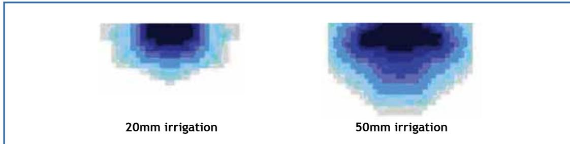
**Figure 3: The influence of the amount of water applied on the wetted volume of a soil**
